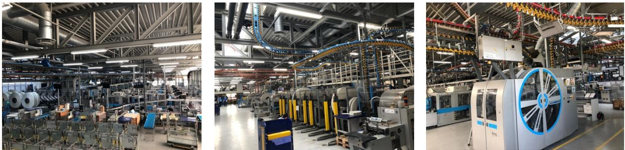
The newspaper printing plant of NZZ Media Services AG in St. Gallen-Winkeln is now equipped with Ferag mailroom technology. Two MultiSertDrum are the centre of attention. The bundles are formed by six MultiStack compensating stackers.
